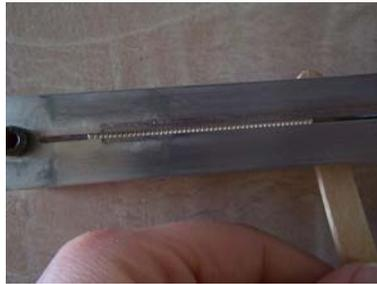
Attach the holder cover with the screws provided. Push the coil all the way down to the stopper with a popsicle stick.
