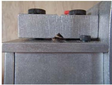
It is set-up similar to a table saw, with a reversible shield that fits on top of the blade to act as a guide for the coil being cut.
