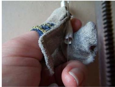
Because the teeth on the saw blade are facing down towards the handle, you will only cut the metal when you are pulling the handle towards you.
