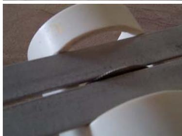
The blade should be mounted so that the teeth are going counter-clockwise.
