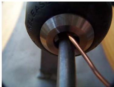
Insert the mandrel into the chuck and tighten it so the mandrel will not fall out.
