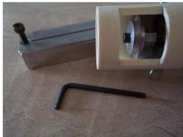
And the Koil Cutter, which includes a blade, arbor, cutter guide, coil holder and an allen wrench.
