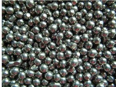
Stainless steel shot is used for the final polish in cleaning jump rings.
