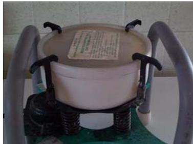
Add liquid burnishing fluid or dish soap (original Dawn) plus water until it is just visible in the media...do not fill the bowl with liquid above the top of the items being tumbled.
