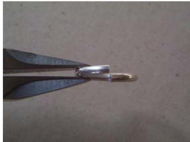
The cut in the top is slightly larger than the blade width used to cut the coil.
