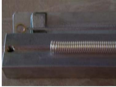
Place the jump ring coil in the groove of the coil holder.
