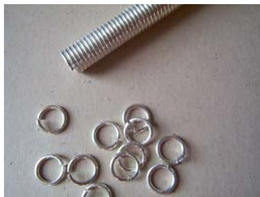
If you find the coil hard to hold while cutting, you may insert the mandrel or a wooden dowel inside for extra support...just be sure not to saw a metal mandrel, as it will break your blade.
