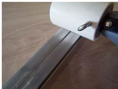
Place the blade guard into the holder top and bring the rotary tool up to full speed.
