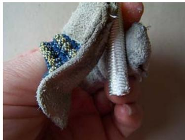
Place some cutting lubricant on the coil and also the saw blade.
