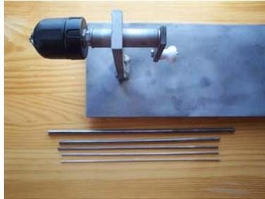
This is my coiling set-up. It consists of a winder and some mandrels\* (metal rods).
