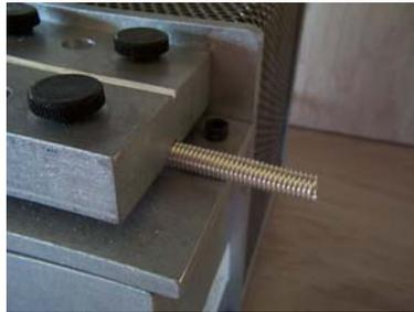
The coil is placed into the guide, and the saw turned on.
