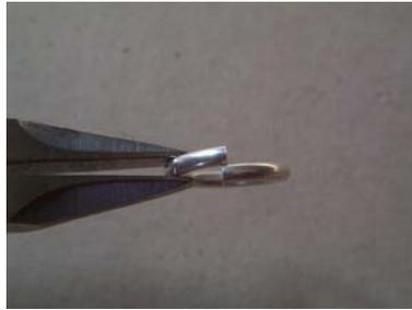
This is known as work hardening the metal. You are rearranging the molecules on the bottom (opposite the cut) of the ring. By rearranging them, they become hard and the jump ring will not pull apart as easily.
