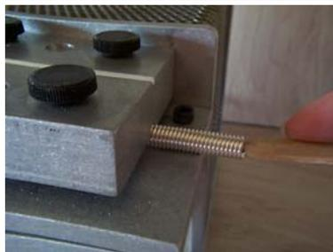
The coil gets pushed over the blade with a popsicle stick, and the rings come out the other side.
